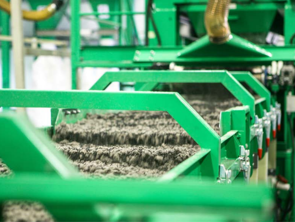
TIRE RECYCLING LINE 1 double line (6 T/h) or 2 lines (3 T/h)
