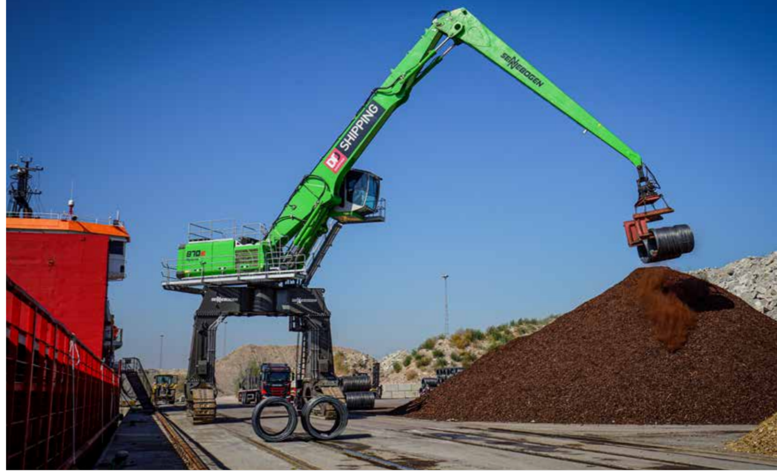
870 R crawler gantry - coil handling; Belgium 870 R Raupenportal - Coil-Handling; Belgien
