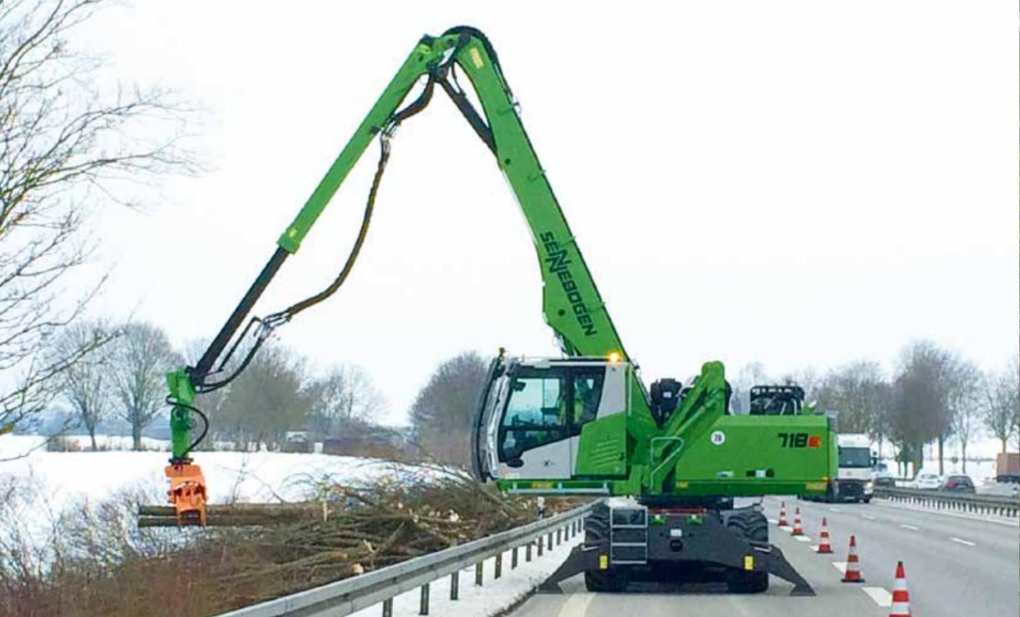
718 – safe cutting-free of routes with cutting head thanks to long reach of 13 m; Germany
