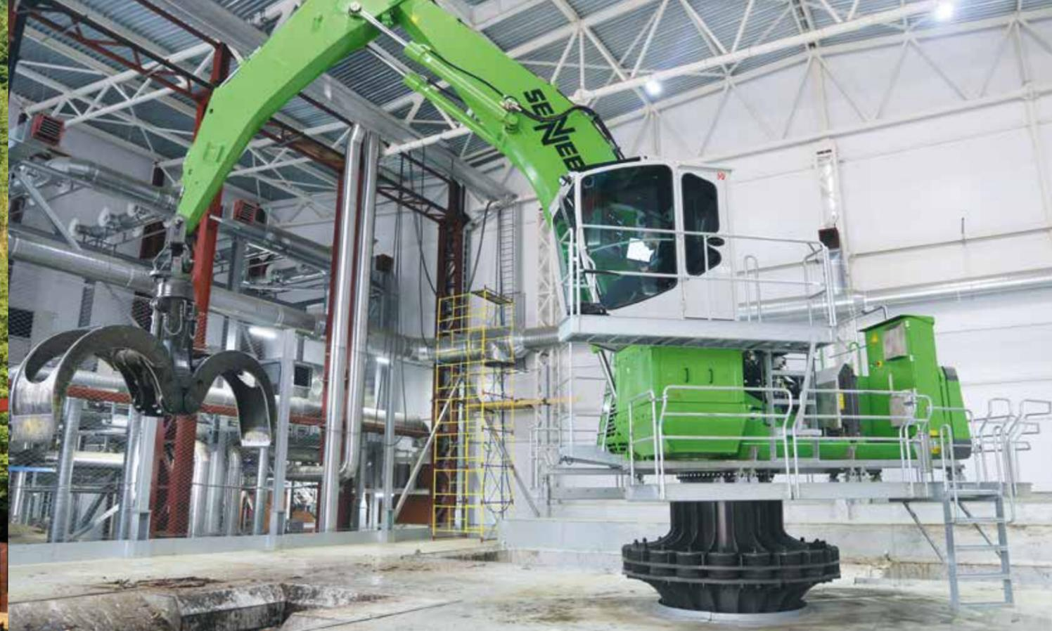
835 Electro - stationary machine with elastic bearing in timber processing; Russia
