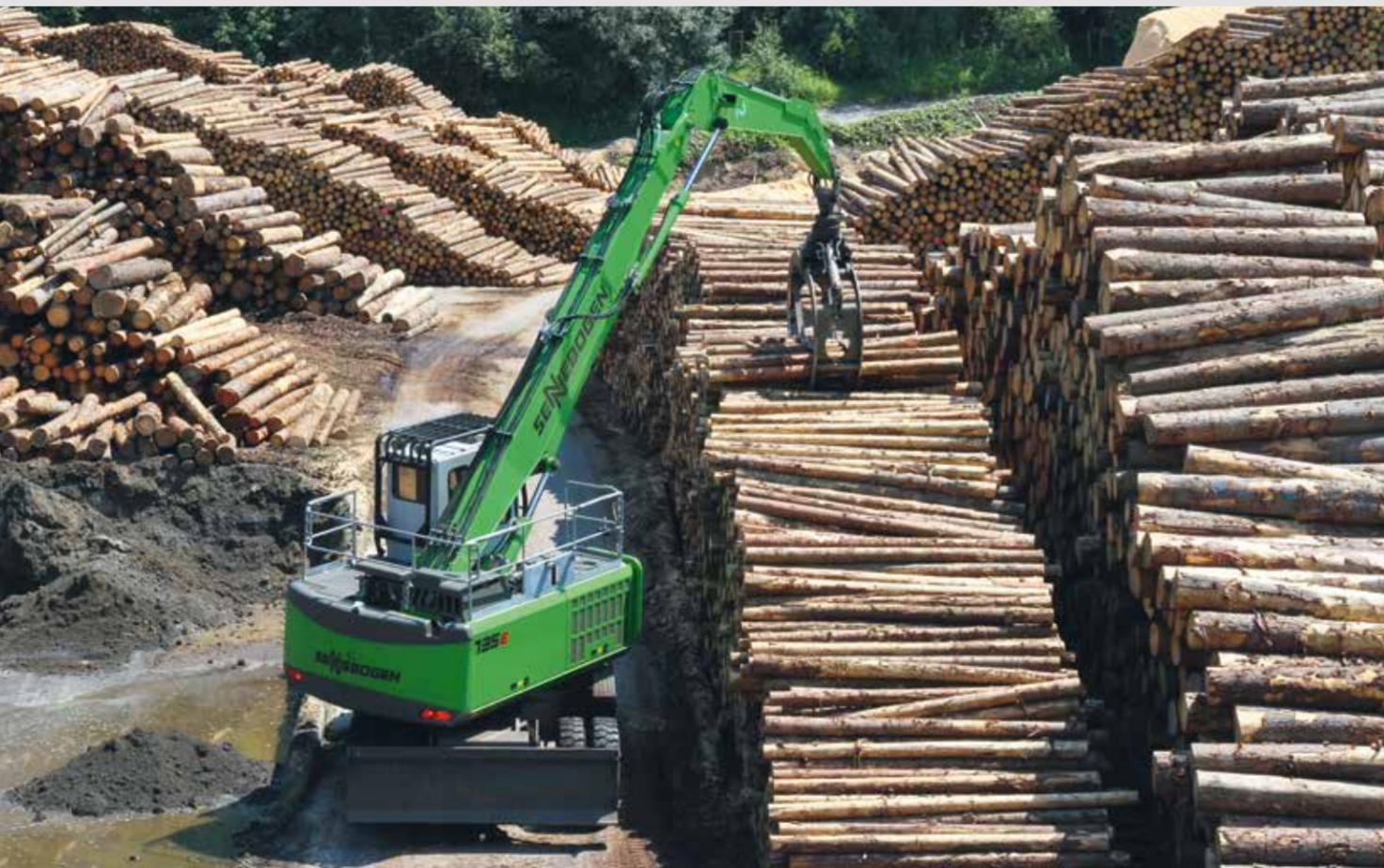
735 M-HD – Pick & Carry in narrow alleys without manouevring in reverse; Austria
