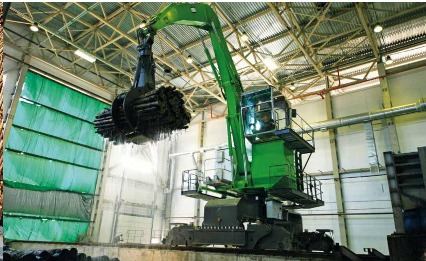
835 Electro - machine with rail gantry undercarriage and power supply via conductor bars in timber processing; Russia
