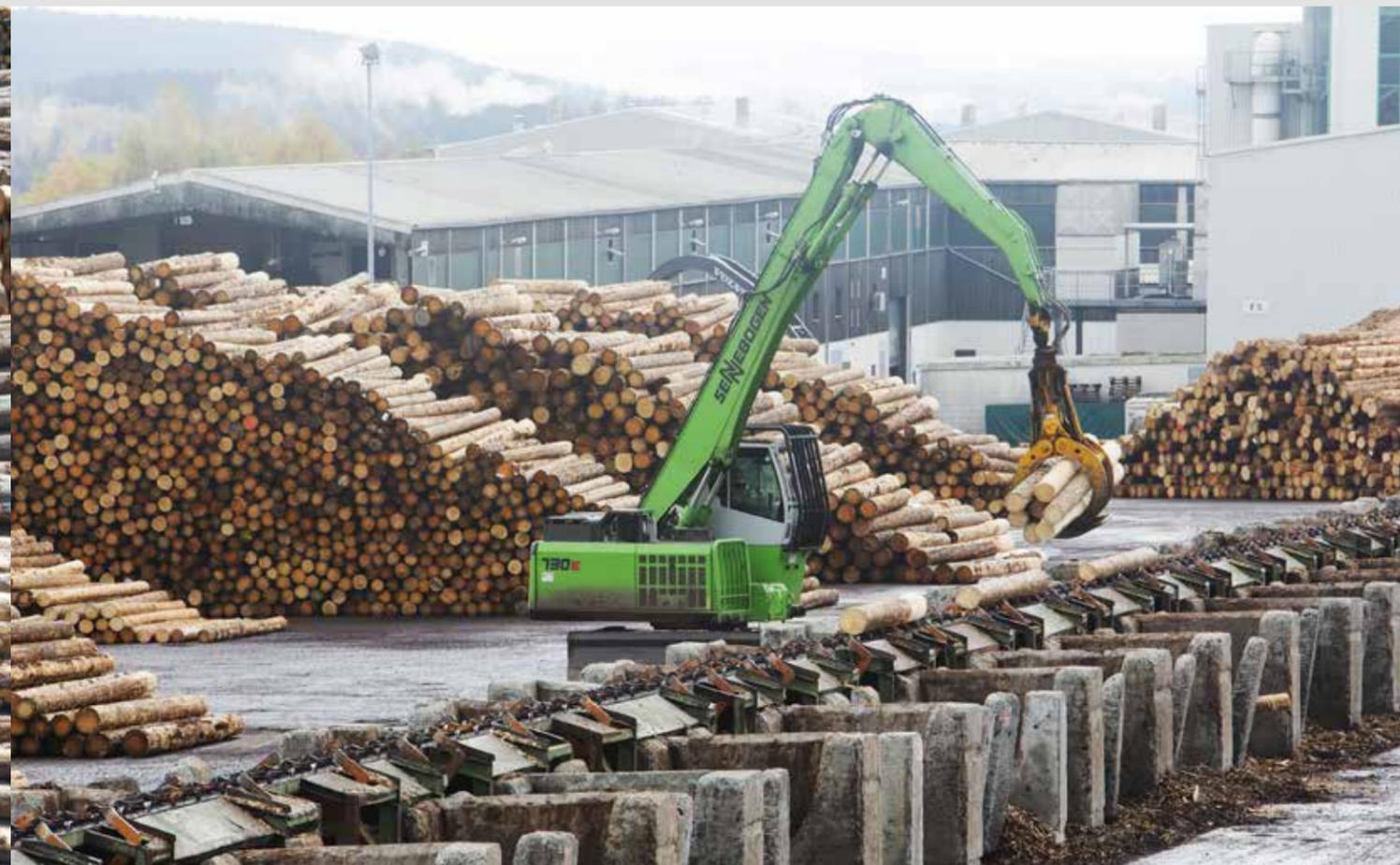
730 M-HD – picking of logs on the sorting line parallel to the driving direction; Germany
