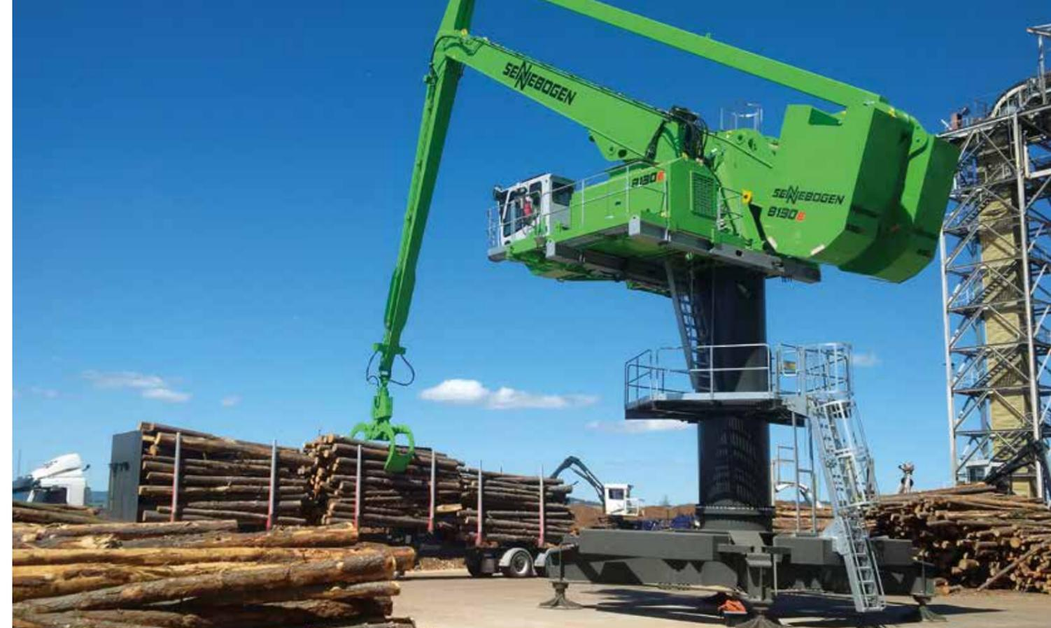
8130 Balancer stationary – handling of round logs, unloading of trucks, process feeding; Australia
