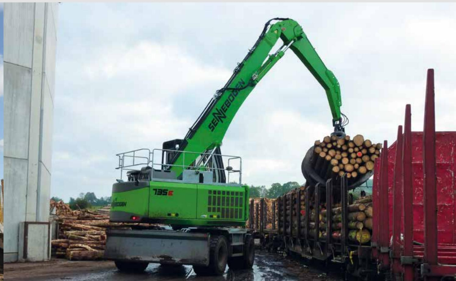
**735 M-HD** – loading / unloading of trains; ideal position of center of gravity by rear linkage of boom
