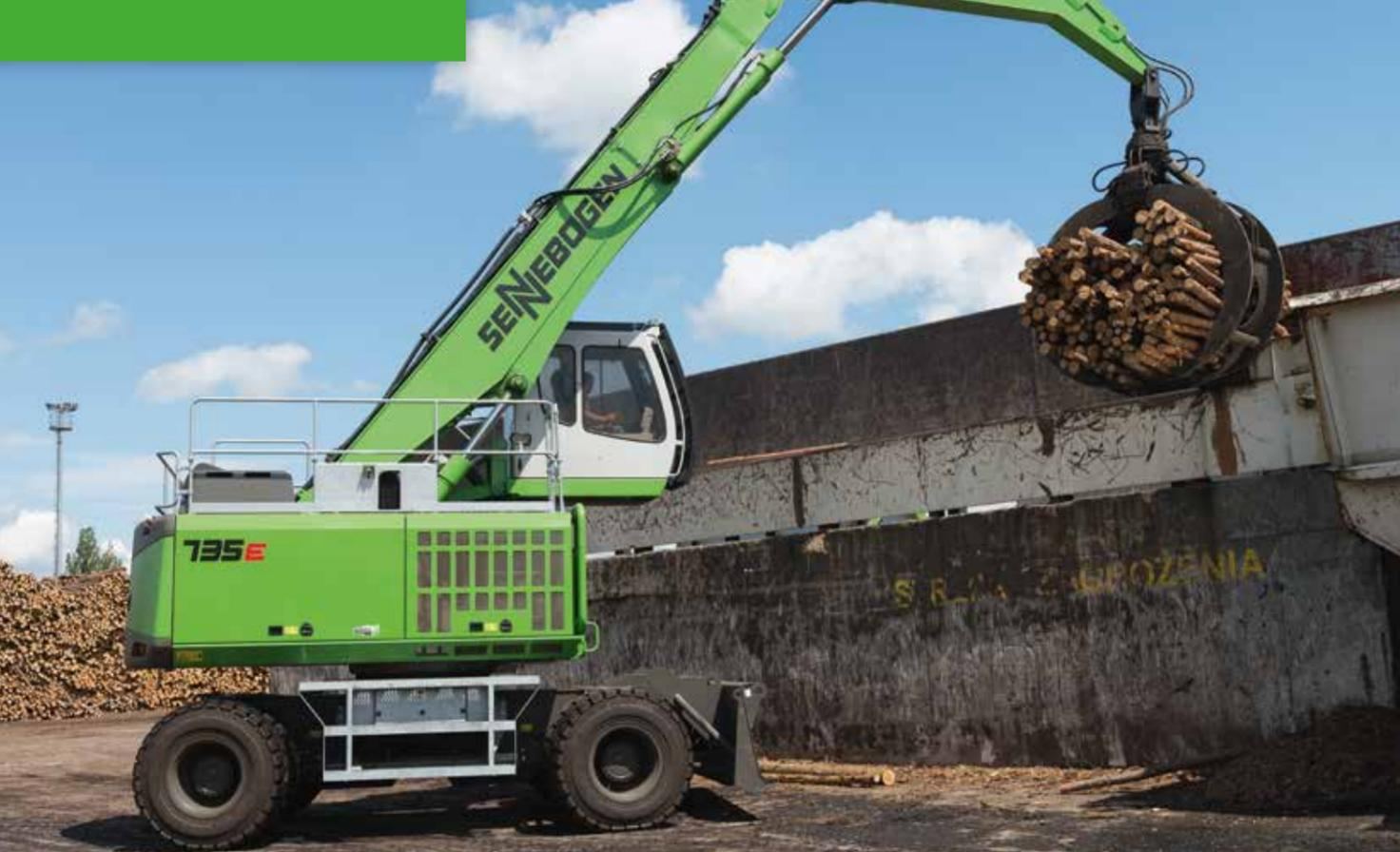
**735 M-HD** – feeding a table rack incl. elevating cab; Poland
