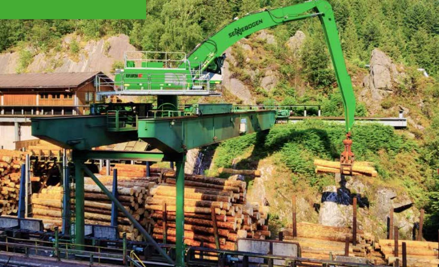
835 Electro - build-up machine on rail carriage and semi-portal for effective storage yard logistics; Germany
