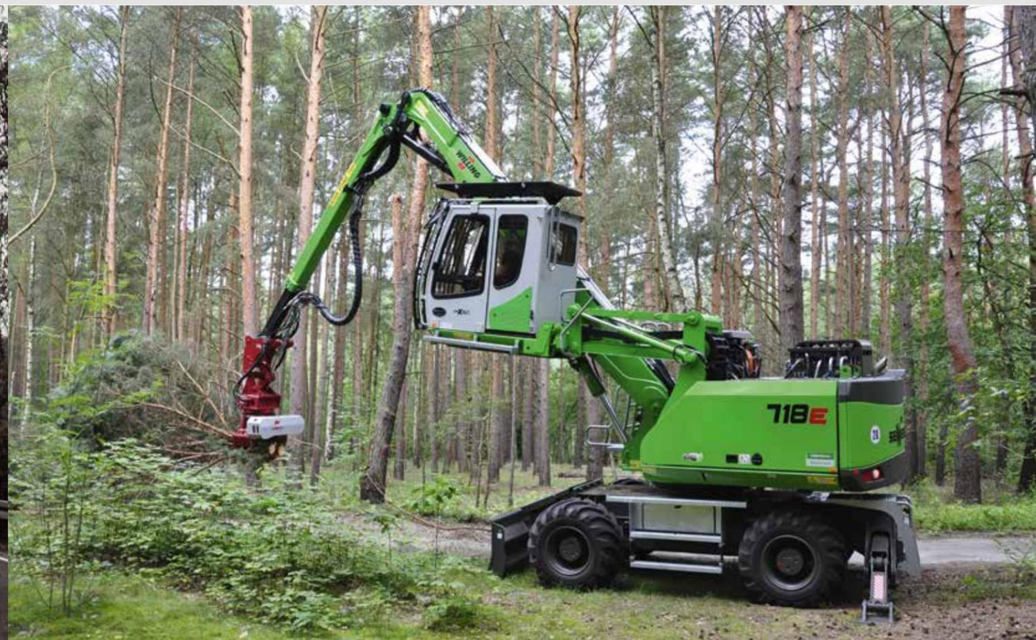
718 – safe cutting-free of routes with grab saw thanks to long reach of 13 m; Germany
