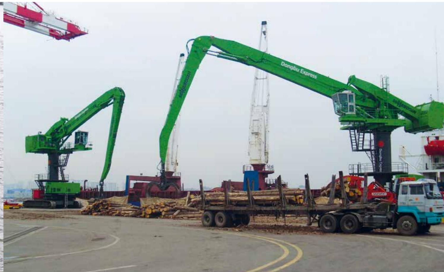
880 EQ - 2 machines with pylon and crawler undercarriage, electric drive and powerpack for independent travel; South Korea
