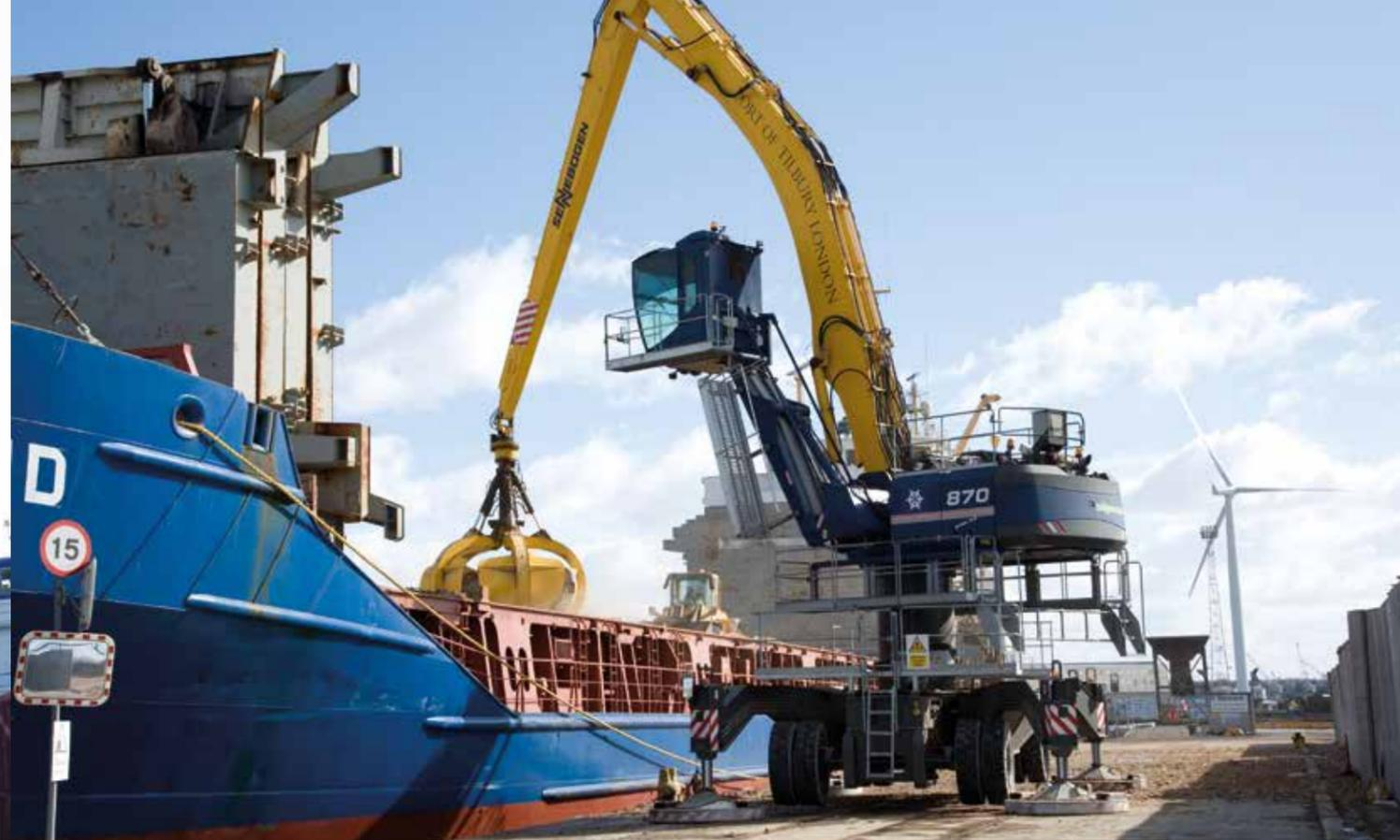
870 M - most rigid undercarriage for large volume wood chip handling, Mastercab with skylift cab elevation; England
