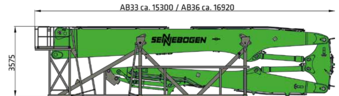
3-PART DEMOLITION BOOM INCL. TRANSPORT FRAME APPROX. 25 T TO 28 t
