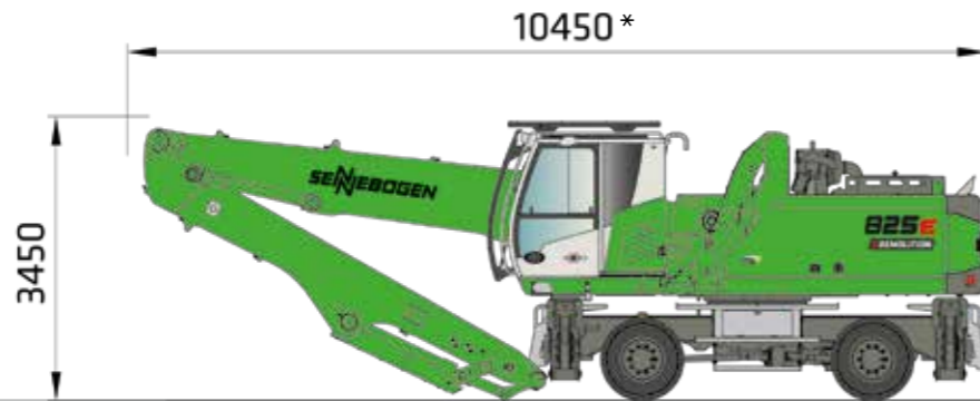
825 DEMOLITION WITH MP26 UNDERCARRIAGE AND K12 ULM EQUIPMENT, HYDRAULICALLY ELEVATING MAXCAB, TILTABLE UP TO 30° AND FULLY HYDRAULICALLY UNLOADABLE COUNTERWEIGHT (OPTION), OPERATING WEIGHT APPROX. 29.5 t
