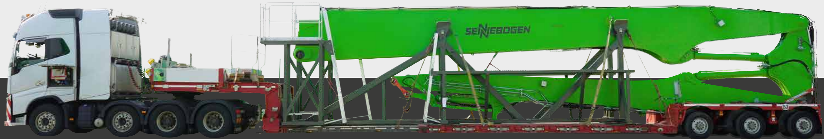
Transport of the three-part equipment in the transport frame (870 Demolition: standard, 830 Demolition: optional)
