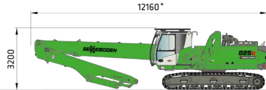
825 DEMOLITION WITH T31/350 UNDERCARRIAGE AND 2-PART K14 ULM EQUIPMENT, HYDRAULICALLY ELEVATING MAXCAB, TILTABLE UP TO 30° AND FULLY HYDRAULICALLY UNLOADABLE COUNTERWEIGHT (OPTION), OPERATING WEIGHT APPROX. 38 t
