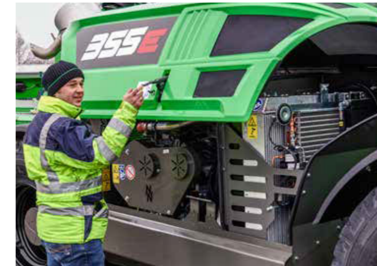
Spacious access to the engine compartment with just one handle. The side plate of the engine nacelle can also be removed.
