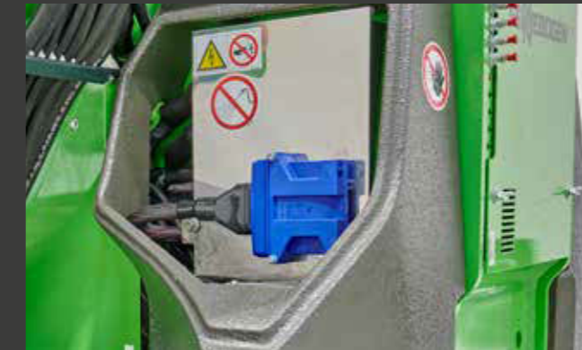
5 Optimum access to the main fuse box with integrated overview plan.
